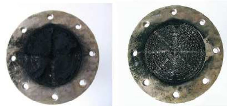
Fig. 4 Metal DPF before and after NTP regeneration
